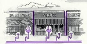
In situations where water is turned off and drainage pipes (specifically P-traps) are empty, the pipes can potentially carry fumigant from one structure to another. Inform your inspector if the water is shut off in the structure to be fumigated.
